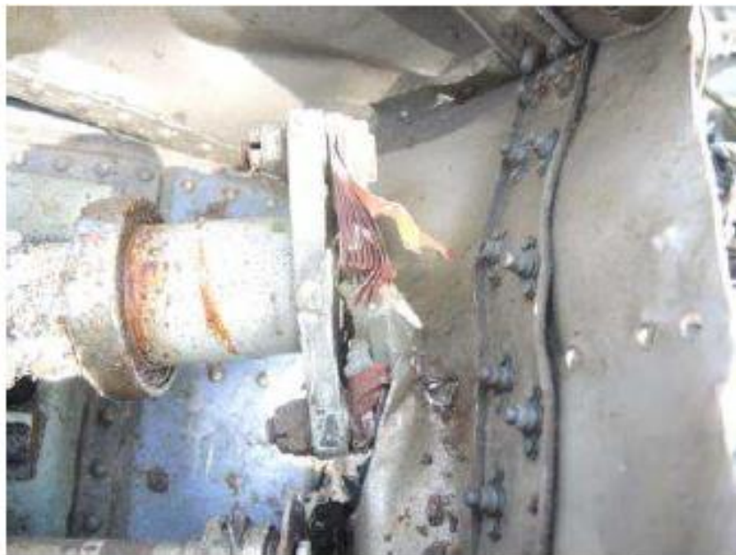
Flexible coupling between the front drive shaft and the centre drive shaft
