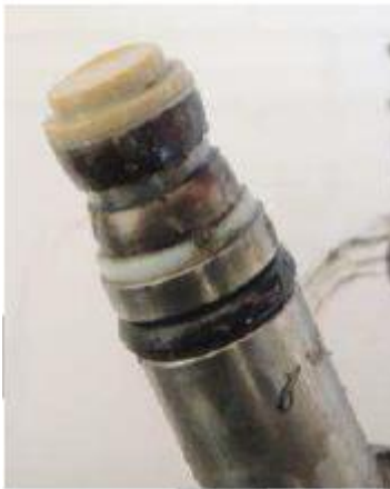
Electrical magnetic plug
