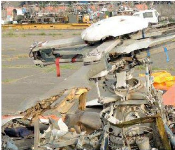
The fragment of the black blade attached to the rotor head
