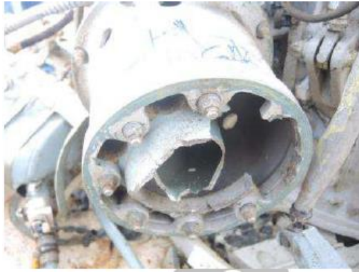
Part of the coupling linked with the main gearbox
