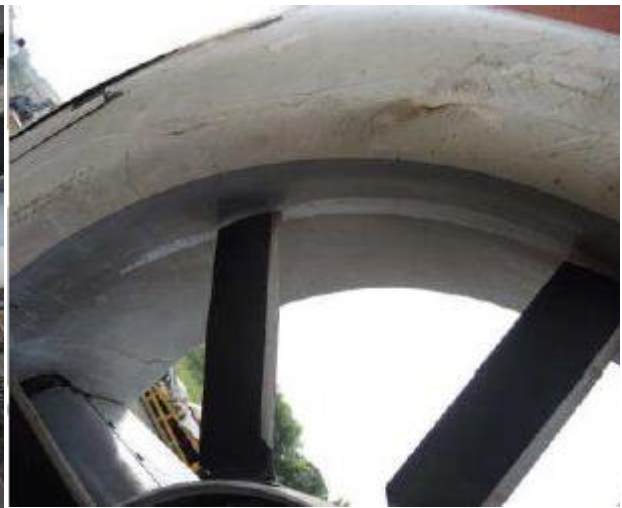
Scuffing identified on the fenestron duct
