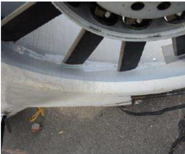
Scuffing identified on the fenestron duct
