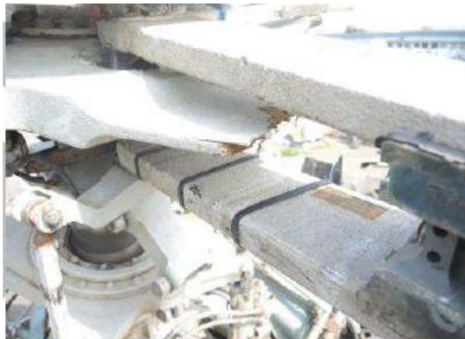
The star arm attached to the fractured black blade
