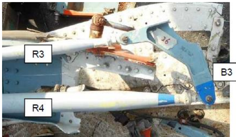
Broken bellcrank B3
